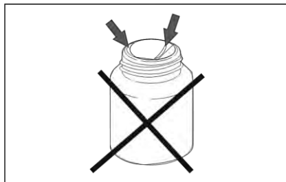
Wax seal on the cartridge damaged
