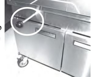
**To avoid overfilling the drain pan, drain only 1 vat at a time. Overfilling the drain pan may cause slippery floors, which may result in personal injury.**
