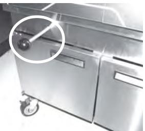
**To avoid overfilling the drain pan, drain only 1 vat at a time. Overfilling the drain pan may cause slippery floors, which may result in personal injury .**
