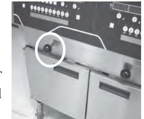
5. Once vat is filled, display may show "IS POT FILLED?" "YES NO". Make sure vat is full and then press button for YES and fryer returns to normal operation. If vat is not full, press NO and oil pumps for an additional 30 seconds.
