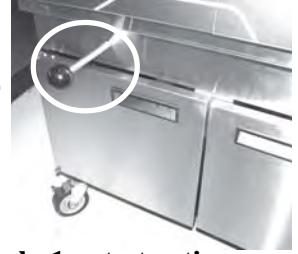
**To avoid overfilling the drain pan, drain only 1 vat at a time. Overfilling the drain pan may cause slippery floors, which may result in personal injury.**
