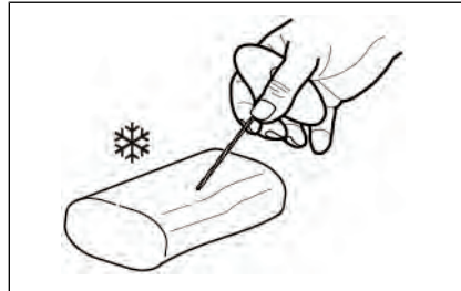
Image: Drilling an insertion duct with a hand drill
