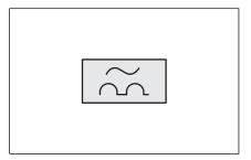
Image: RCD switch type A circuit symbol
