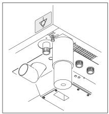
Image: Connecting the potential equalization
