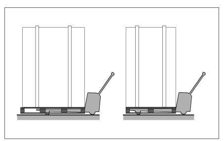
Image: Lengthwise and crosswise transport on pallet
