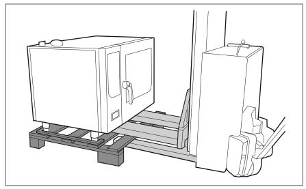
Image: Lifting the unit off the pallet
