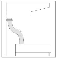
Image: Connecting the exhaust air line
