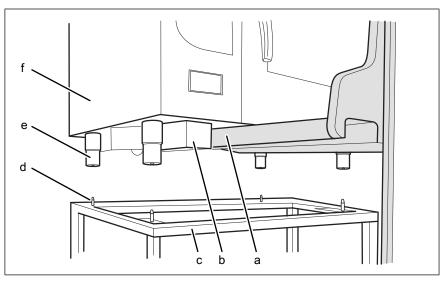
Image: Setting up the unit on a base frame
