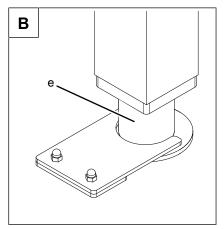
Image: A: Position of floor plate; B: floor plate glued to the floor
