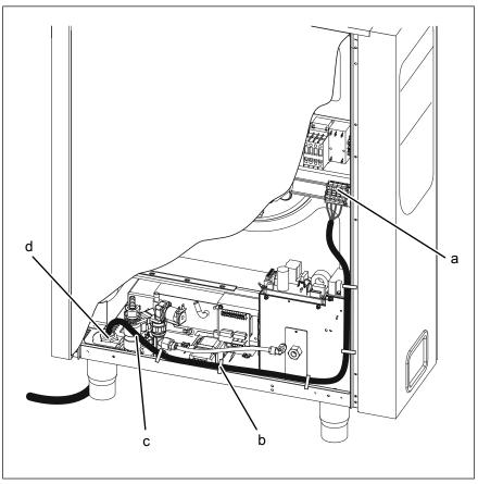
Image: Connecting the electrical connection line
