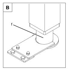
Image: A: Position of floor plate; B: floor plate bolted to the floor
