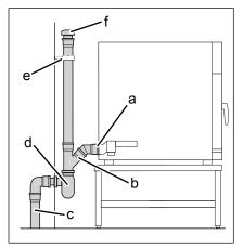
Image: Waste water line to a permanent connection
