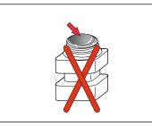
Image: Wax seal on the cleaning cartridge damaged
