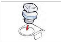
Image: Insert the cleaning cartridge in the holder
