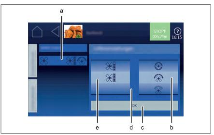
Image: Setting the fan speed and direction of rotation
