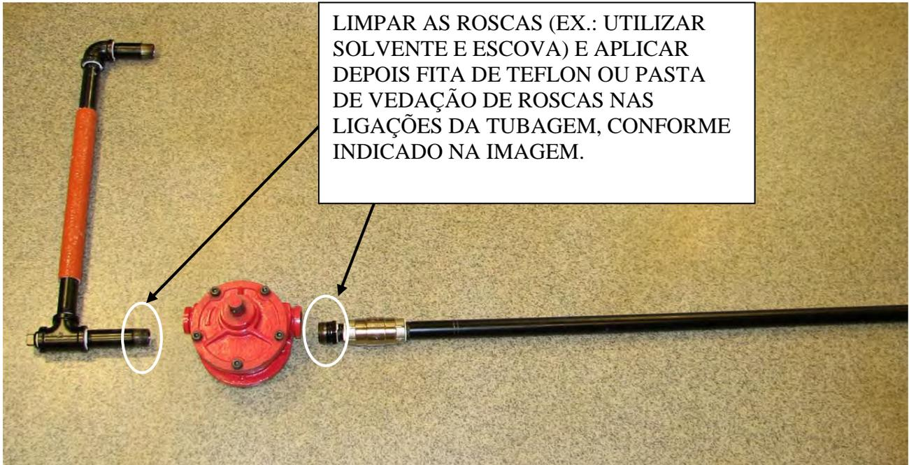
LIMPAR AS ROSCAS (EX.: UTILIZAR SOLVENTE E ESCOVA) E APLICAR DEPOIS FITA DE TEFLON OU PASTA DE VEDAÇÃO DE ROSCAS NAS LIGAÇÕES DA TUBAGEM, CONFORME INDICADO NA IMAGEM.
