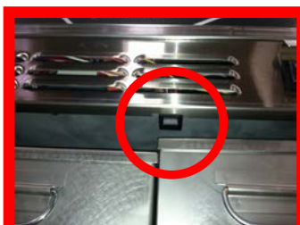
High Limit Reset Switch
